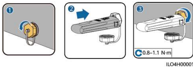
Figure 3-9 Installing a Smart Dongle
